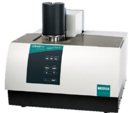
LFA 467 HT HyperFlash ® Suitable for thin samples and high thermal conductivity materials
